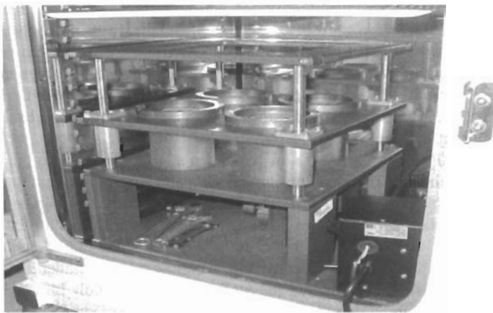
Figure 3: Equibiaxial Strain Device (EBASD) with four membrane holder rings. The device is placed in an incubator during operation.
