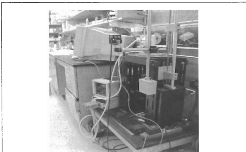
Figure 7: Our photo of the Mechanical Tester (MT) seen from a different angle. Grouped to the left (of a person standing in front) is a PC, computer screen, keyboard and mouse. Various components of the MT are connected to the computer through an acquisition board. The acquisition board is used to sample and synchronize force and position data using LabView software; in addition, the signal from the load cell transducer is transmitted through an amplifier signal conditioner. The servomotor of the MT receives analog input from the load cell transducer and communicates signal outputs to the PC computer. The CCD camera is connected to the PC computer through another specialized acquisition board, images are collected using the imaging software Inspector .
