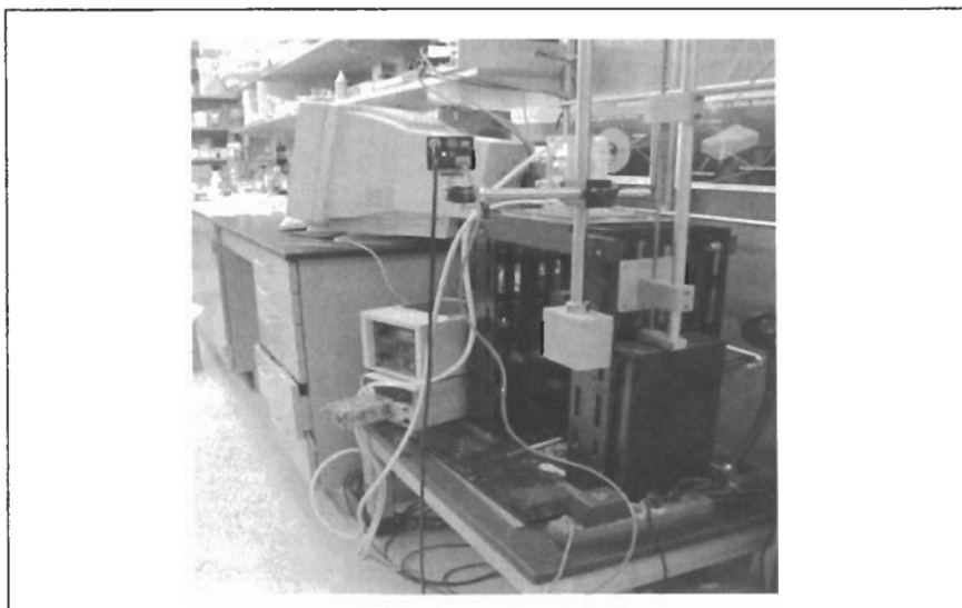
Figure 7: Our photo of the Mechanical Tester (MT) seen from a different angle. Grouped to the left (of a person standing in front) is a PC, computer screen, keyboard and mouse. Various components of the MT are connected to the computer through an acquisition board. The acquisition board is used to sample and synchronize force and position data using LabView software; in addition, the signal from the load cell transducer is transmitted through an amplifier signal conditioner. The servomotor of the MT receives analog input from the load cell transducer and communicates signal outputs to the PC computer. The CCD camera is connected to the PC computer through another specialized acquisition board, images are collected using the imaging software Inspector .
